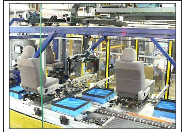
Automation equipment with several servo motor applications.
