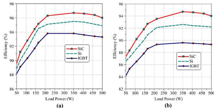
Efficiency comparison for 50 V input at a 20 kHz, b 50 kHz switching frequency (1)
