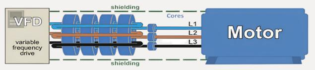
Because of the size and weight of Nanotech<sup>TM</sup> cores, it may be necessary to clamp and mount the cores to the wall of the drive, or other area between drive and motor. It is not required, but does make the system look more esthetic, and provides support for heavier cores. Available are special made brackets, with threaded rod, that can easily clamp and mount the cores to a structure.
