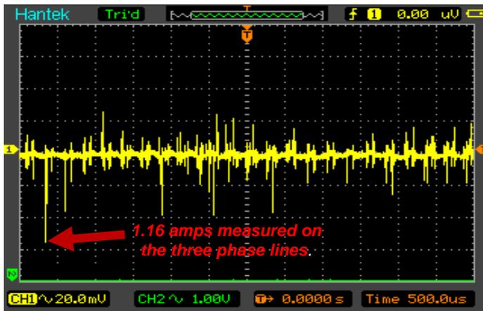
Phase leads with cores installed:
