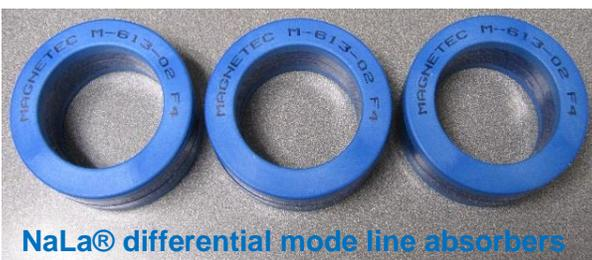
*The inductive absorbers are an inductor and common mode choke designed to absorb damaging current before it gets to the motor. The inductive absorber cores are placed in series over the three power conductors between the VFD and motor, and the NaLa® differential mode cores are mounted around each of the three conductors individually. These products have been in use in Europe for some time but are just now available in the USA.*
