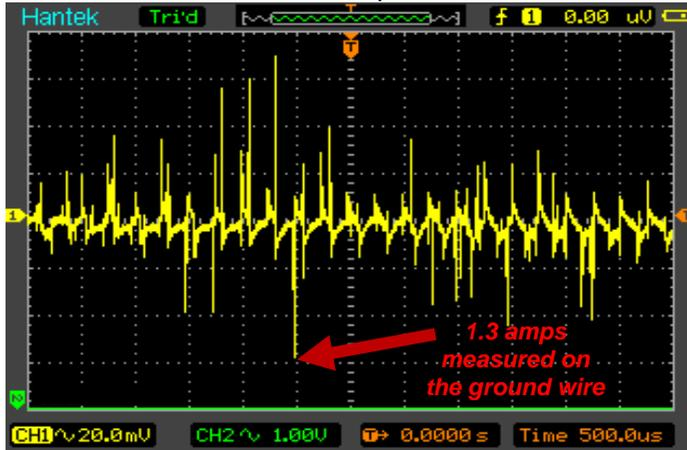
Ground lead with cores on phase leads:
