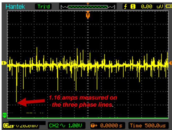
We operated a 5 horsepower motor and VFD on our shop dynamometer and recorded the common mode and stray currents to ground.
