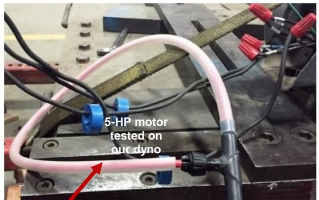
*Rogowski coil installed around the 3-phase lines to the electric motor to measure the amount of current "not" flowing back to the 3-phase lines*
