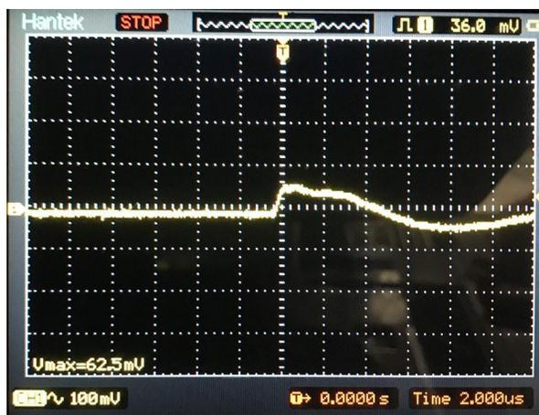
*With CoolBLUE and NaLA installed on cables near the VFD*
